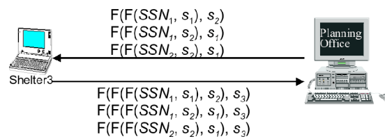
Figure 61. Round 3 of de-duplication. Shelter 3 receives the current mixed values of the UIDs that were originally contributed by Shelter 1 and Shelter 2.
