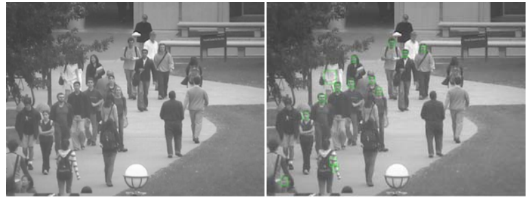
Figure 1. Image captured from publicly available webcam on left and with automated face detection on right.
